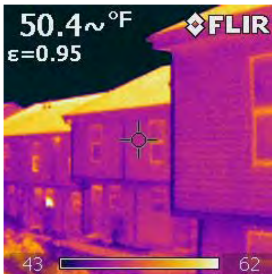
This infra-red elevation image shows heat loss at the window frames. The roofs appear to be a warmer surface due to solar gain (sun warm-up).
